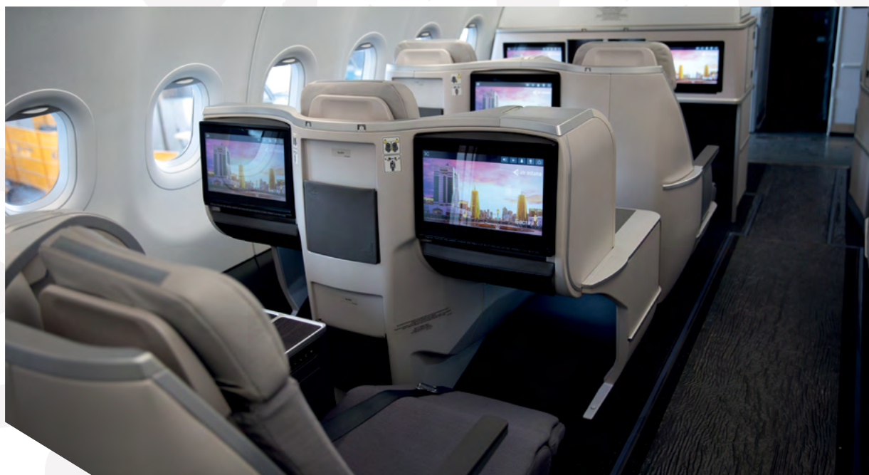
The newly designed business class on the new A321LR, features a variant of Thompson's Vantage seat with a more intuitive seat control mechanism; RAVE IFE and purple and white soft furnishings.
